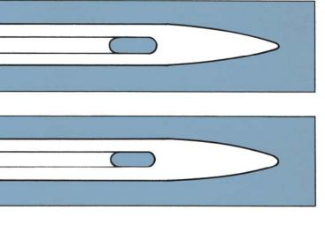
1. The universal ballpoint needle (705H) has a slightly rounded tip; therefore, the needle separates the threads of the fabric. It does not pierce the individual threads which may damage the fabric, resulting in runs or snags. The 705H needle point is the most versatile as it is suitable for knit or woven fabric and is available in sizes 60-120.
