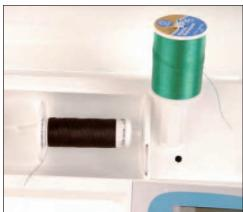
3 Thread guides come in various shapes and forms. The next step is usually a thread guide. It may be a hook design or a button design (a). Drawing thread from the spool, run the thread to the thread guide, which is closest to the spool of thread (b).
