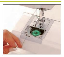
Once the sewing machine is threaded, the needle is lowered (a) and raised by turning the balance wheel to catch the bobbin thread and bring it through the throat plate (b). See pages 70–73 for threading the sewing machinge.
