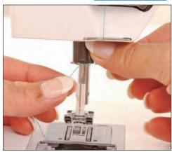
8 You made it! You're at the sewing machine needle. Thread the needle, and place the thread tail under the presser foot toward the back of the machine. Thread the bobbin and bring the bobbin thread up through the throat plate.
