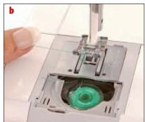
A large variety of sewing machines have a bobbin case. They mount differently from machine to machine. Most have a latch that releases the bobbin case from the machine.
