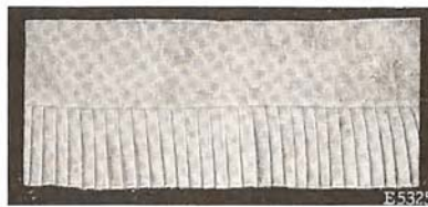
FIG. 139. SAMPLE OF PLAITING AND SEWING TO THE GARMENT IN ONE OPERATION
