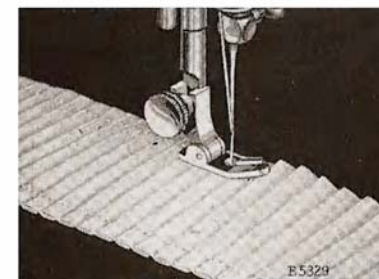
FIG. 143. SEWING PLAITS FLAT WITH THE PRESSER FOOT
