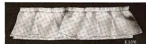
FIG. 127. SAMPLE OF RUFFLE MADE AND APPLIED IN ONE OPERATION
