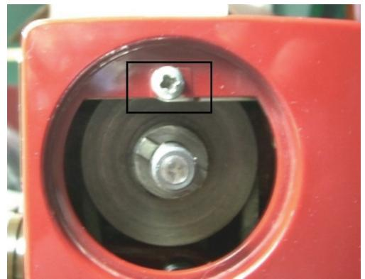
A screw located directly under the bobbin winder thread guide screws directly into the white plastic back cover.
