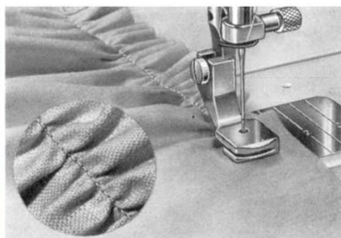
40 93 019. Presser foot for gathering. Gather the material as you sew, the harder thread tension, the stronger gathering.
